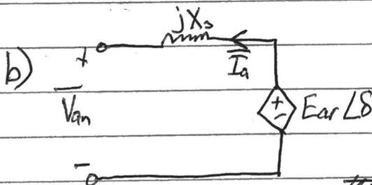
$$E_{ar} L \delta = j X_s \bar{I}_a + V_{an} L 0$$
