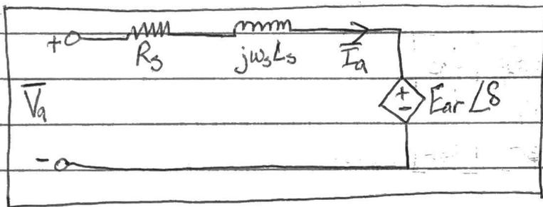
$$E_{ar} = \frac{\omega_s M I_r}{\sqrt{2}} \quad \therefore \text{excitation voltage, dependent on } I_r$$
